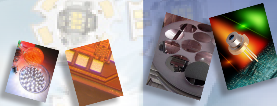
Pictures (above) from left to right: LED bulbs from LEDtronics; GigOptix's GX3110 chip; MOCVD reactor at Finisar; and Sanyo DL-8142-201 IR laser.
