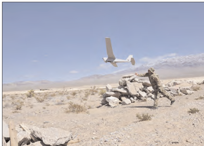
Figure 7. Launch of AeroVironment’s Puma AE small unmanned aircraft that has achieved 9 hours flight using Alta solar power.
