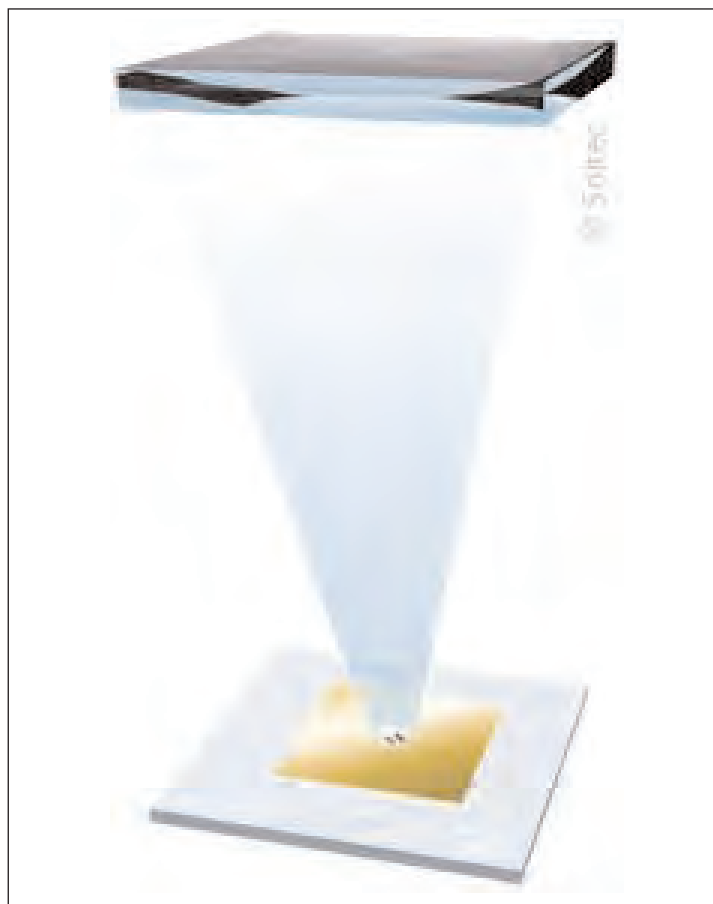
Figure 3. Schematic diagram of SOITEC's concentrated photovoltaic module.
