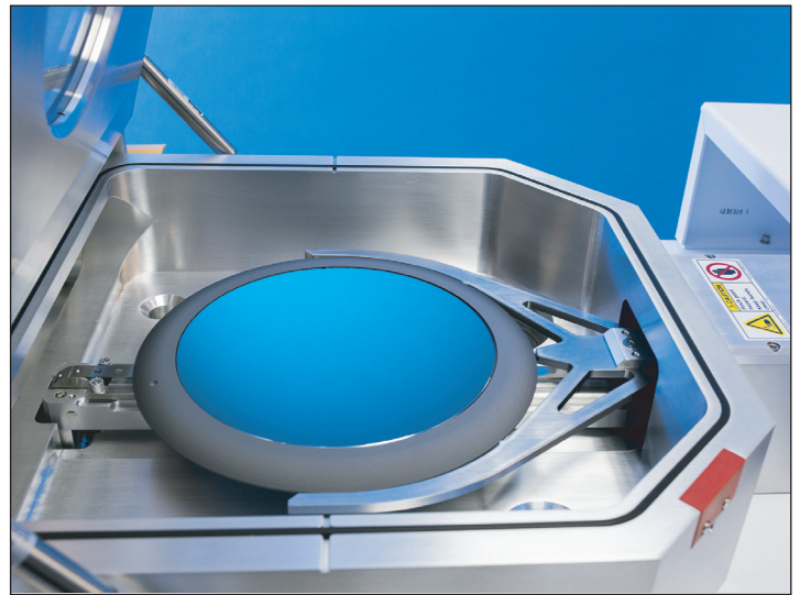
Wafer in Veeco's Propel PowerGaN MOCVD system.
