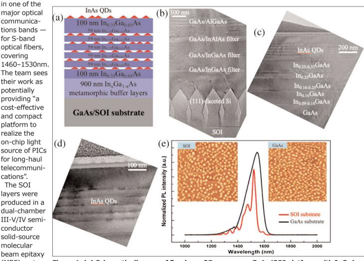
(MBE) system: Figure 1. (a) Schematic diagram of five-layer QDs grown on GaAs/SOI platform with InGaAs metamorphic buffer layer. (b)-(d) Cross-sectional transmission electron microscope images silicon dioxide of GaAs-on-SOI template, InAs/InGaAs metamorphic structure, and InAs QDs, respectively. (e) Room-temperature PL spectra of five-layer QD structure on SOI (red curve) and GaAs (black curve) substrates. Inset: 1µmx1µm atomic force microscope images of surface QDs.
