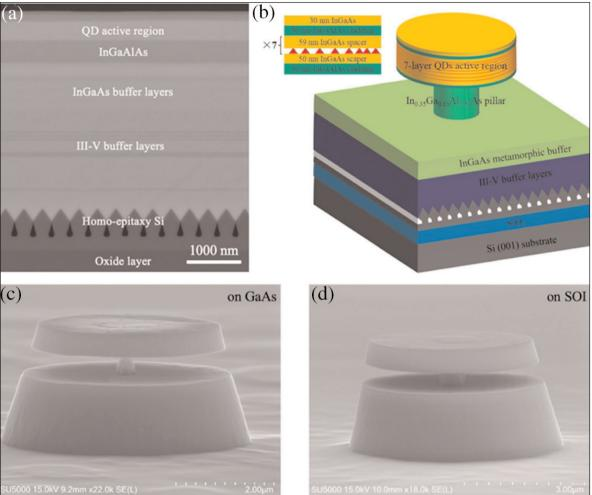
Figure 2. (a) Cross-sectional scanning electron microscope (SEM) image of microdisk sample on SOI substrate. (b) Schematic of microdisk laser. Inset: schematic of active In<sub>0.35</sub>Ga<sub>0.65</sub>As layers: region. (c), (d) Tilted SEM images of microdisk lasers on GaAs and SOI platforms. a 14nm 425°C cap
