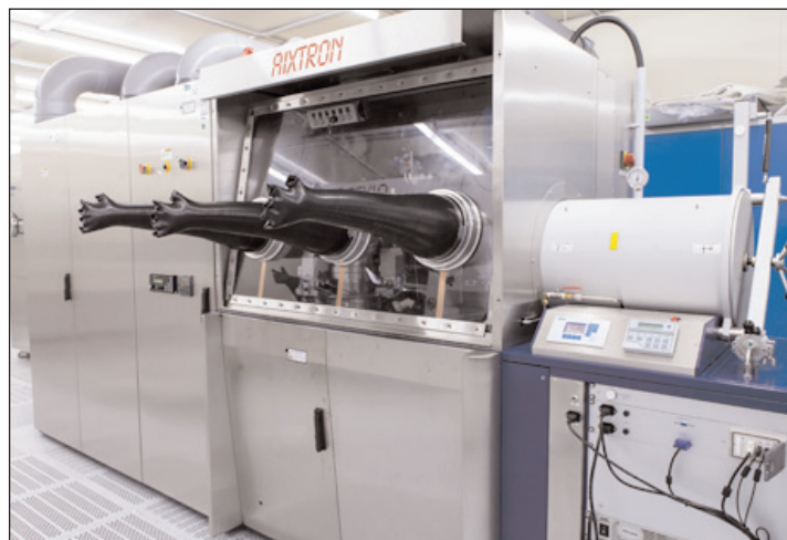
Fraunhofer IAF's MOCVD system has been modified to enable the growth of AlScN with sufficient quality and productivity for industry.
