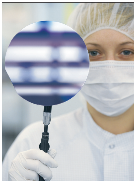
OSRAM high-performance LED chips based on InGaN technology are fabricated on wafers with a diameter of 6 inches.
