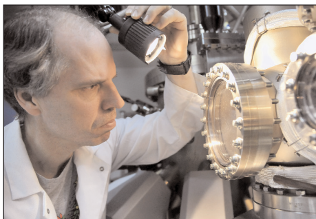
Bennett transfers samples into an MBE system prior to growth of InAs quantum wells for high-speed, low-power-consumption transistors.
