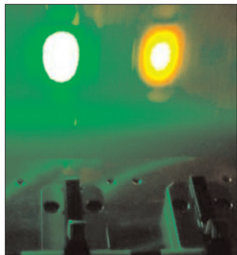
Projected laser light (561nm and 594 nm) from compact laser modules.
