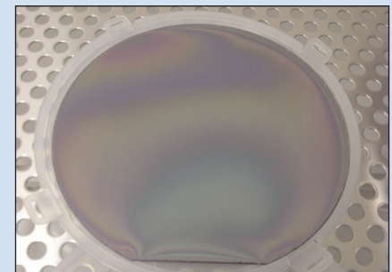
p82 AZZURRO Semiconductors' 150mm GaN-on-silicon template wafer, ready for shipment.
