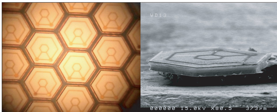
Honeycomb chips before separation (left) and SEM image of separated honeycomb chip (right).
