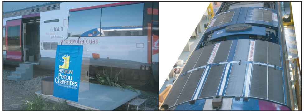
SNCF's Photovoltaic Train (left) and Ascent Solar's modules applied to roof.
