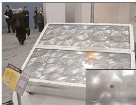
Sharp's CPV panel and (inset) solar cell beneath the Fresnel lens. Credit: M. Kanellos/CNET News.com
