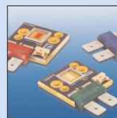
p55 A bar with ten terahertz lasers, the first room-temperature electrically pumped semiconductor sources of coherent terahertz radiation.
