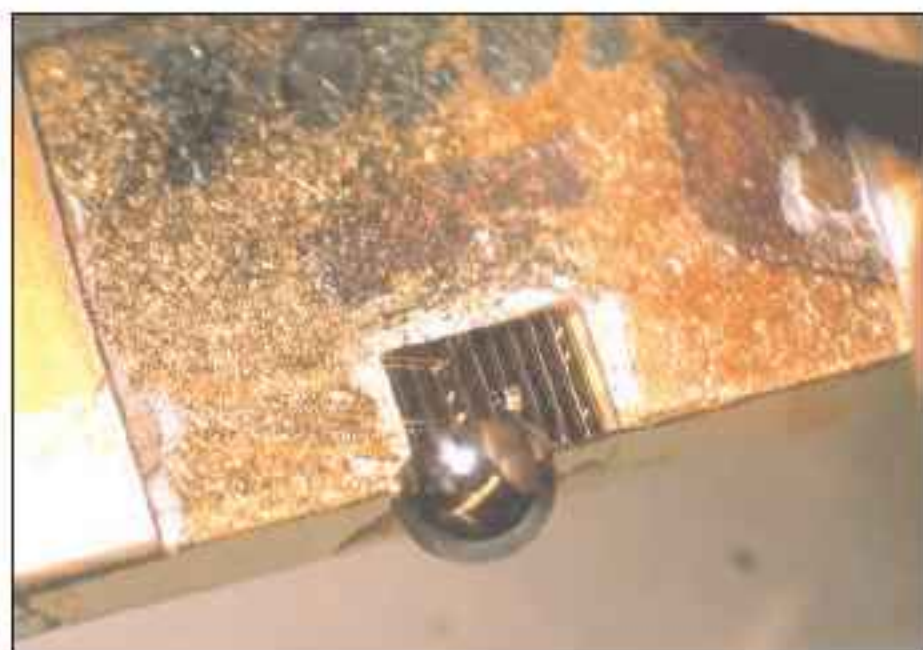
A bar with ten THz laser sources. One of the lasers is connected to the contact pad (on the left) by two thin gold wires. A 2mm-diameter silicon hyper-hemispherical lens is attached to the facet of the device to collimate the output. The emission frequency is 5THz (a wavelength of 60 \mu\text{m} ). Photo: Capasso Lab, Harvard SEAS.
