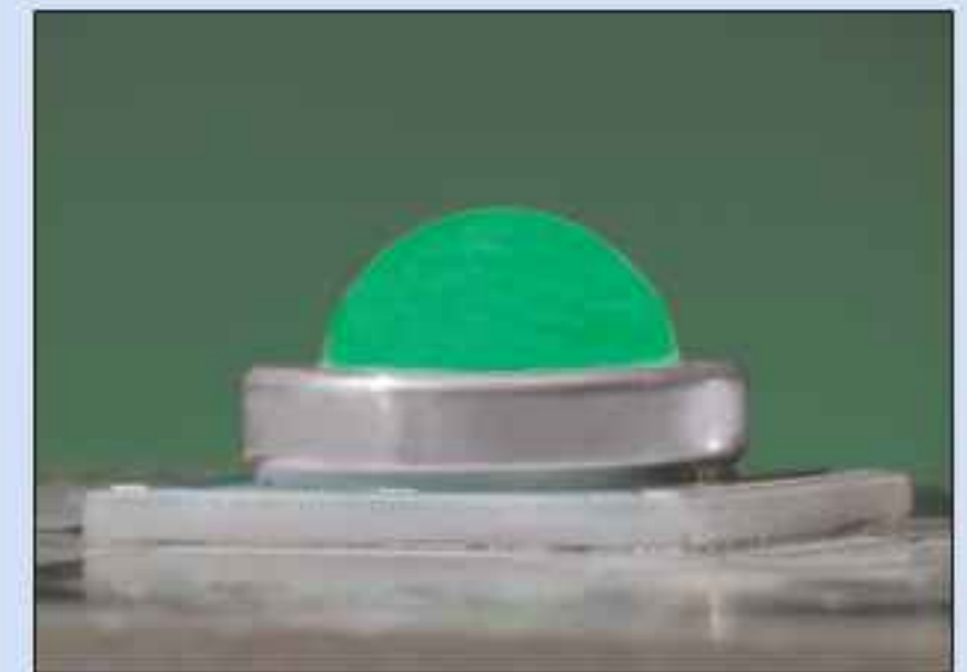
p36 Cree has added to its existing white XLamp XR-C LED with new blue, green, amber, red-orange and red versions to offer a full range of colors.
