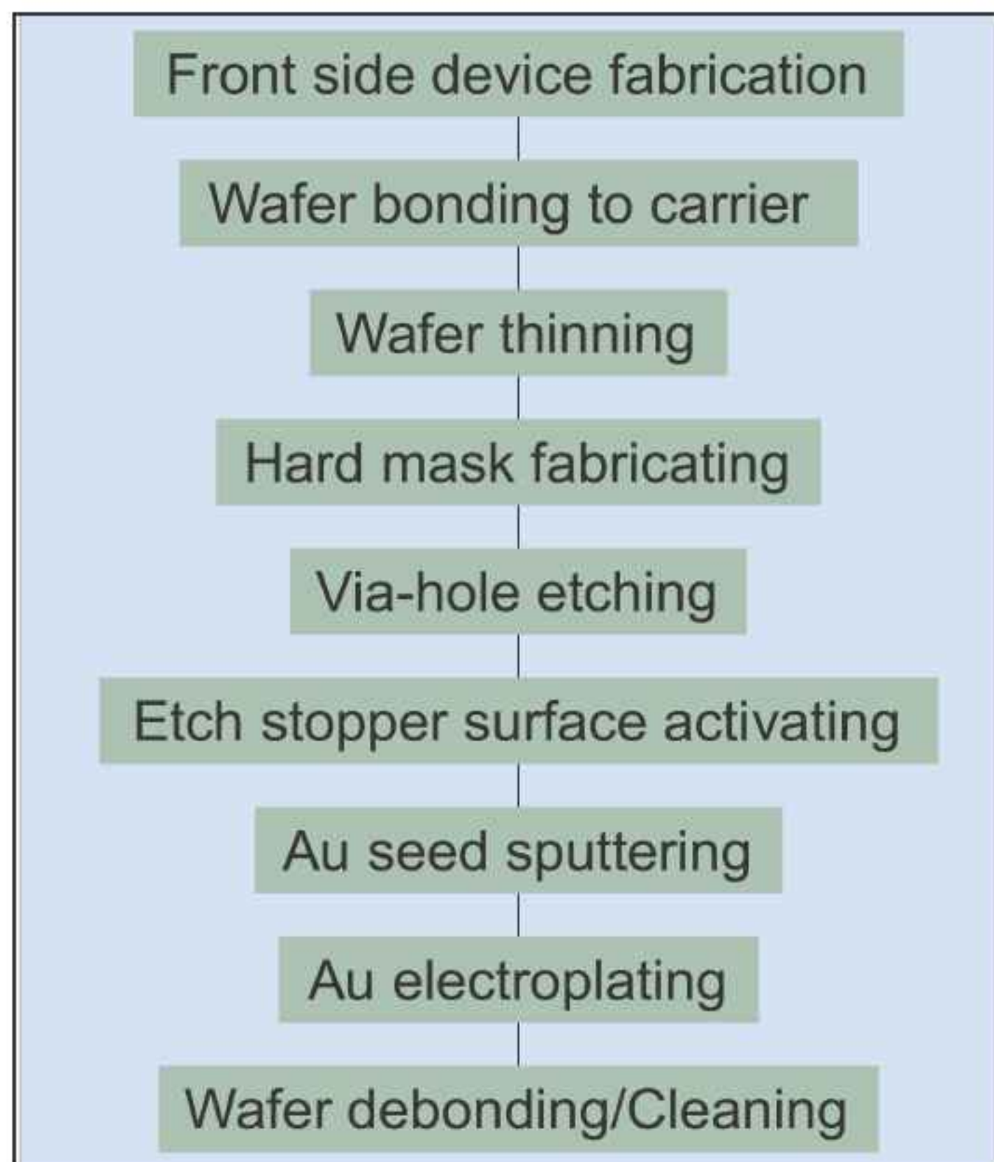
Figure 3. Fujitsu process for SiC via-hole etch.
