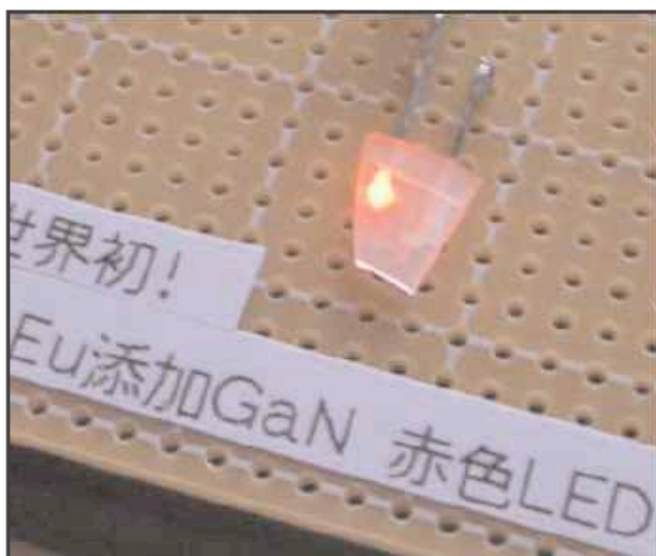
Osaka University's Eu-doped GaN LED, which emits red light with a wavelength of 621nm.
