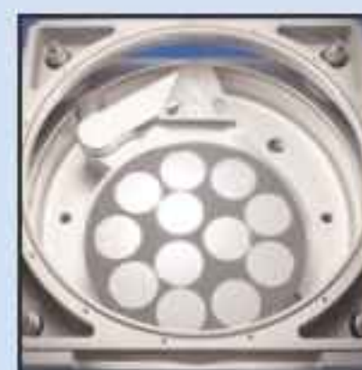
Cover: Veeco's K465i MOCVD reactor (launched in January), showing 4" sapphire wafers, removable carrier, and automated loading. New techniques that can improve process uniformity aim to boost capital efficiency, lowering LED production costs and driving adoption for solid-state lighting. p87
