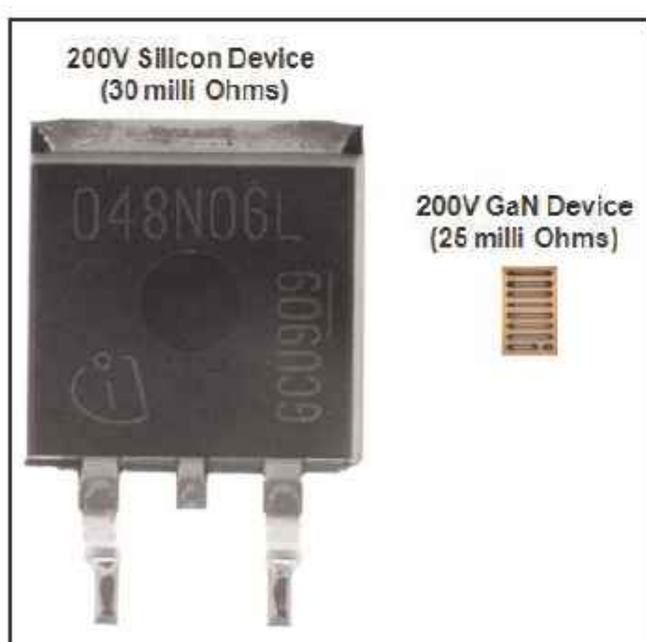
Size of EPC's 200V GaN device compared to equivalent silicon device.
