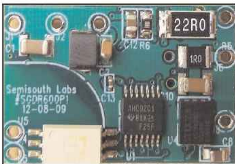
SGDR600P1 reference gate driver for 1200V, 63m \Omega , normally-off SiC JFET.
