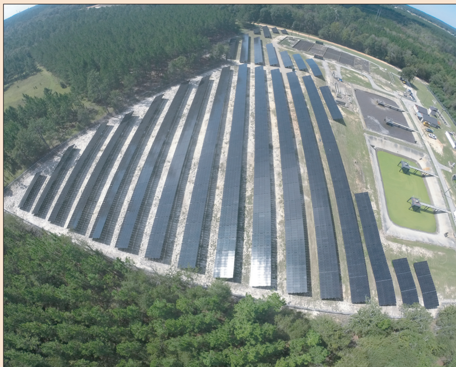
The 1MW solar array at the Vidalia Water Treatment Facility.
