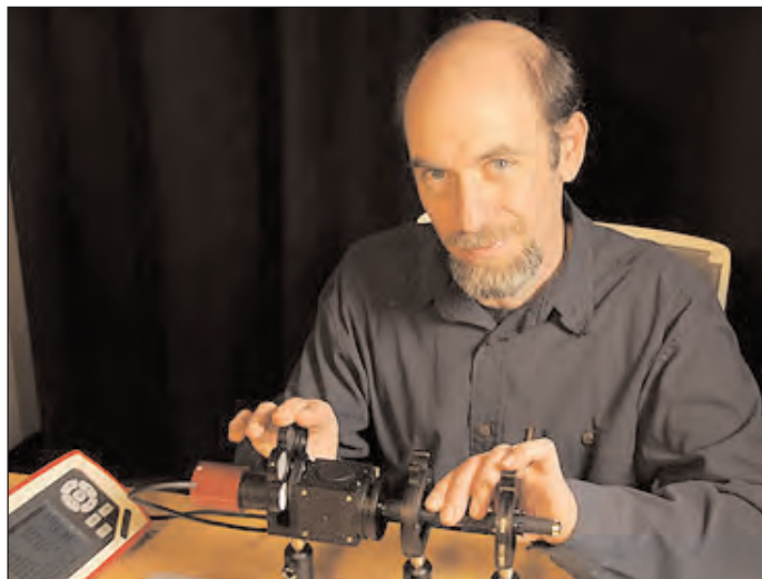
NIST laser safety officer Joshua Hadler and his apparatus for measuring the properties of handheld laser devices.
