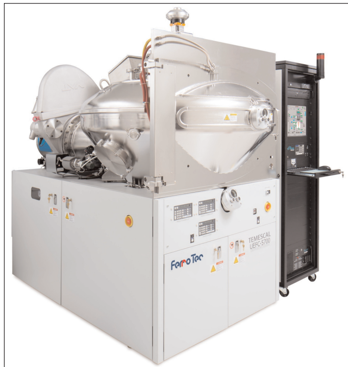
Fig. 1: Ferrotec UF-5700 electron-beam evaporator for the manufacturing of SAW and BAW devices.
