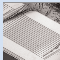
p68 NREL/CSEM's GaInP/Si tandem cell, which has set a record one-sun dual-junction efficiency record of 29.8%.
