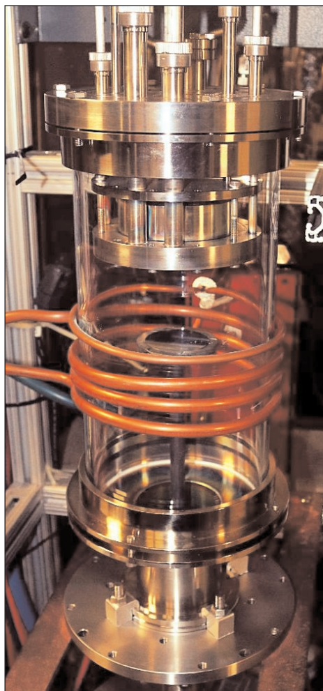
SMI's in-house NanoV CVD reactor with a 2" wafer platter in place — the system can also run a 3" size wafer.
