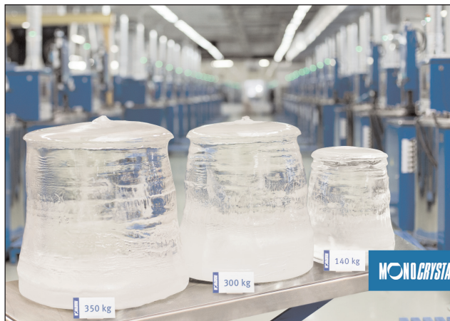
Monocrystal's 350kg KY sapphire crystal (left), next to its 300kg and 140kg crystals.
