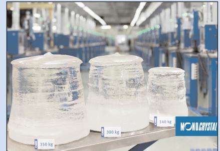
p44 Monocrystal has demonstrated what is said to be the first 350kg Kyropoulos sapphire crystal, here next to the firm's 300kg and 140kg crystals.
