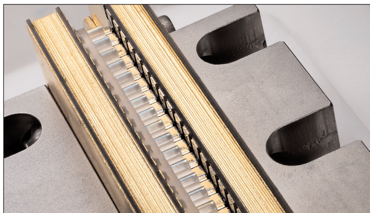
A diode laser stack with lenses, for use as a pump laser in industrial applications.
