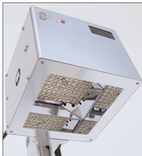
UV-LED irradiation system comprising 120 233nm-wavelength LEDs, for inactivating pathogens or coronaviruses without damaging the skin.
