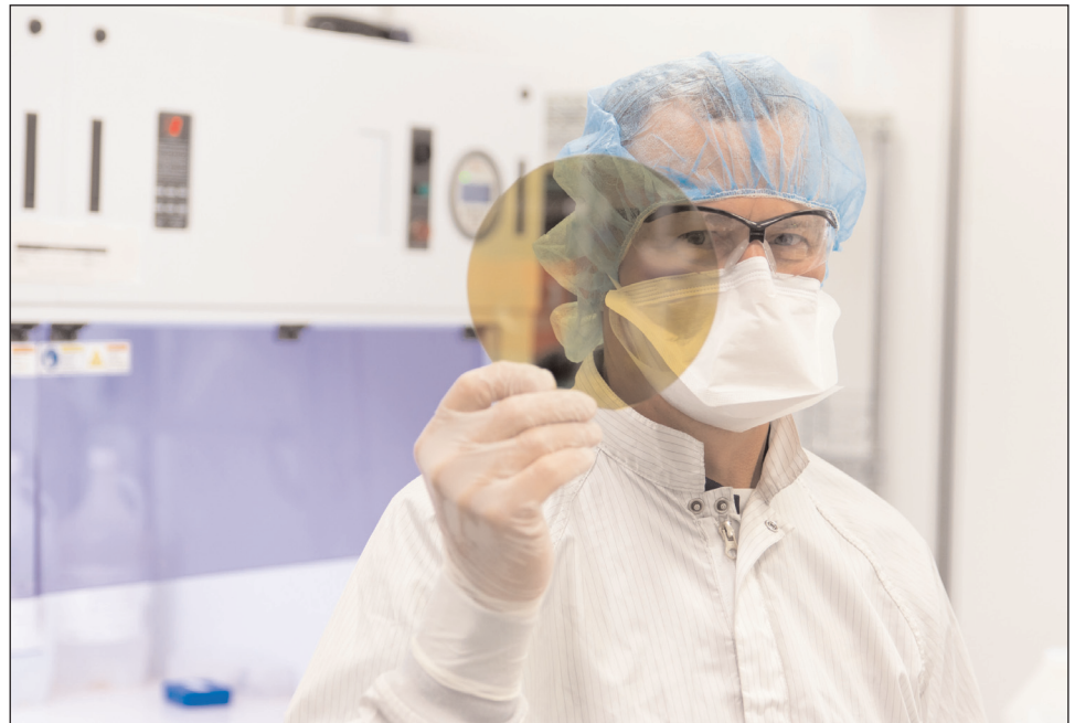
A silicon carbide wafer produced at SK Siltron CSS' Michigan facility. The company plans to expand its Michigan operations to increase production of these wafers, which can be used in power system components for electric vehicles.
