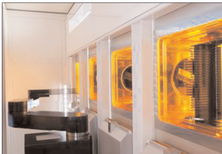
The new VIISa 900 3D hot ion implant system.
