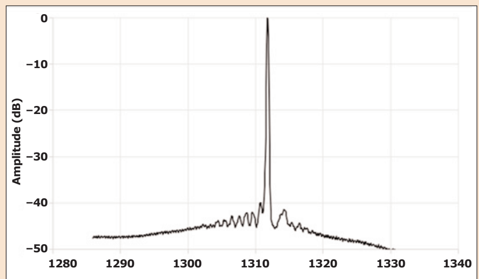
Optical output of new 1310nm photonic-crystal surface-emitting laser, showing side-mode-suppression.
