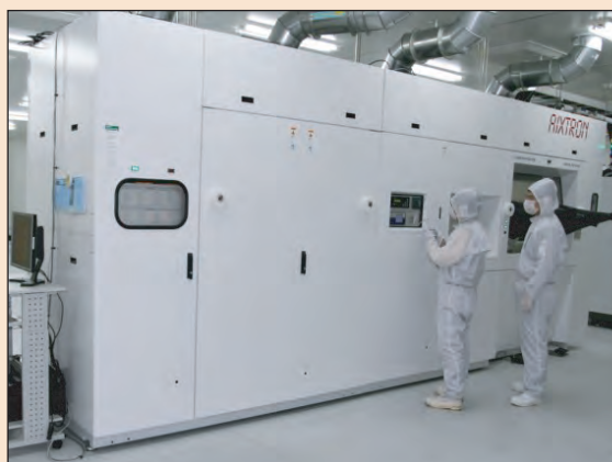
An Aixtron reactor, used for SiC epitaxy.
